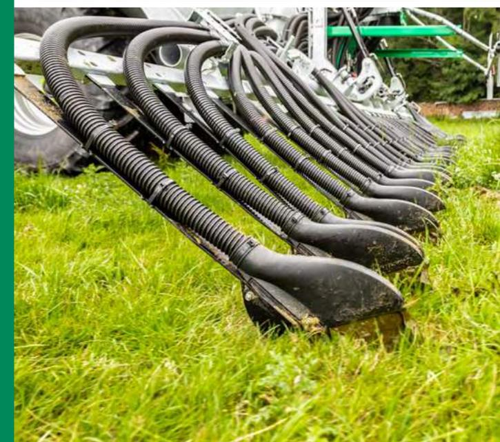
The 43 mm diameter hoses are very flexible and follow the routing on the machine without high tension. The smooth interior surface optimises the flow. The specially developed SAMSON black hoses provide unique UV resistance.
