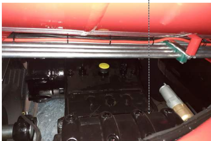
Spulepumpe placeret under tanken
