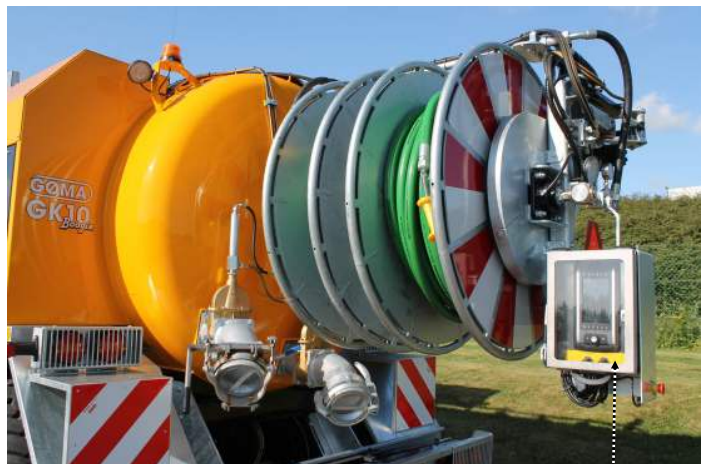
Control panel back with display
