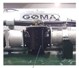
Three-way valve on the side of the carriage for unloading through crane
