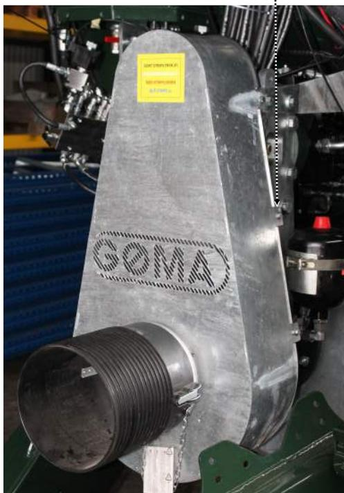
Filling of oil for bearing housing (1.25l max, 1540 engine oil).
