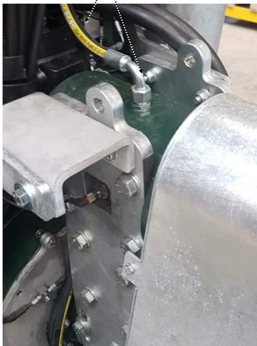
Ventilation hose MUST point upwards.
