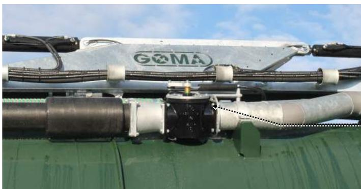
Operation of the three-way valve is carried out from the joystick or the display. See separate manual.
