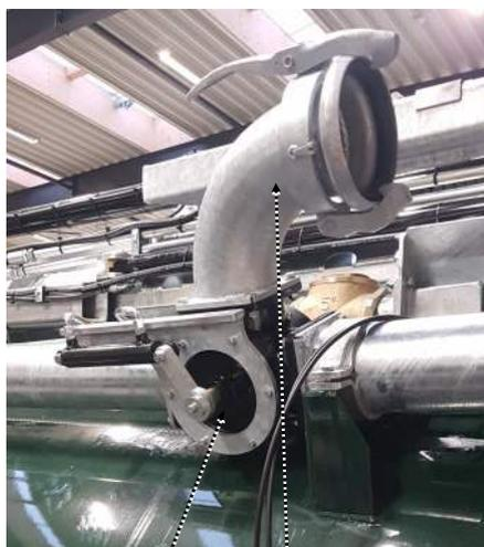
Three-way valve at the back of the tanker for unloading through pipe
