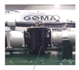
Three-way valve on the side of the carriage for unloading through crane
