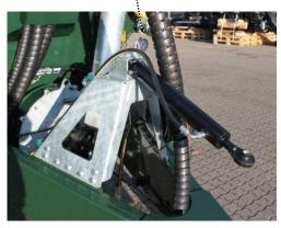
Three-way valve in the back of tanker
