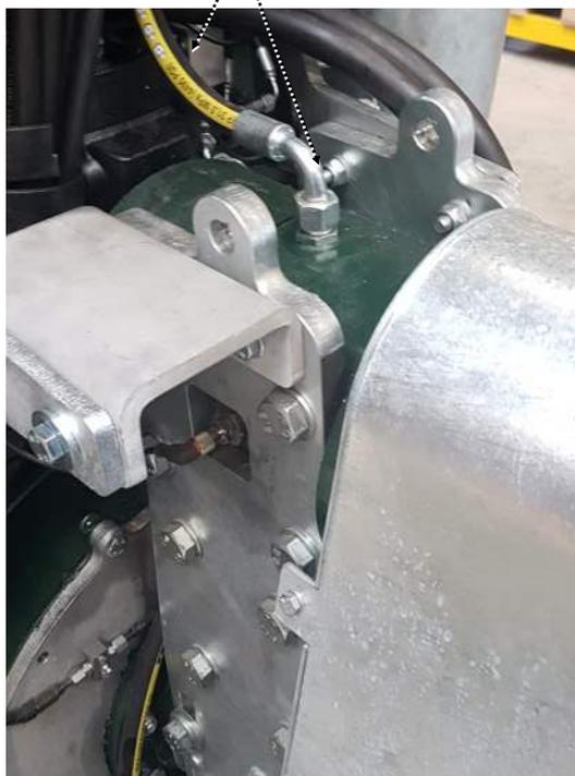
Ventilation hose MUST point upwards.
