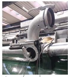
Three-way valve at the back of the tanker for unloading through pipe
