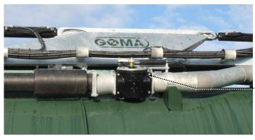
Operation of the three-way valve is carried out from the joystick or the display. See separate manual.
